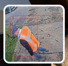
A person approaches the machine from behind, the sensor detects the per son by marking it with a red square.
