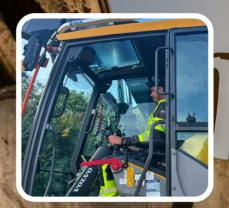
MEDguard warns the machine operator with a red light indication in the cabin as soon as the person approaches the machine from behind.
