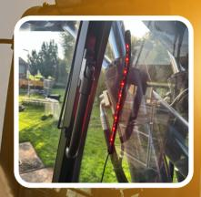
The red Led Indicator is placed within the driver's direct field of view.
